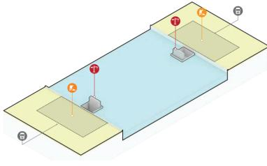
Temporary footing on bank side, and place first truss section
