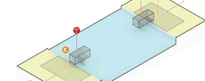
Weld truss sections on bank side as rolling bridge across the river
