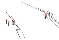
from a barge or the riverbank. The pylons may need to be supported by temporary props. Cable anchors constructed.
