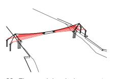
are also transported by barge and hoisted into position in a balanced manner: again a navigational channel is maintained throughout. Once there is sufficient deck hung from the main cables to stabilise the pylons, the temporary props and surrounding cofferdams are removed.
