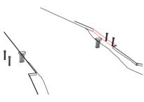
**04.** Land may need to be **05.** Pylons craned into position reclaimed on the south bank to and bolted onto pile-caps, either accommodate access ramps.
