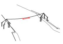
**08.** The first and central deck **09.** The remaining deck segments segment is transported by barge, before being hoisted into position and hung from the main cable: a navigational channel is maintained throughout.
