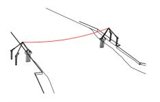
**06.** Pilot cable is cast across the **07.** Using a pulley system on the pilot cable, the preformed main cables are pulled into position and anchored.
