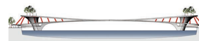
Phase 4. The upper cables connected to the lower deck at the mid point of the span will be tensioned: the structure is in its final position.
