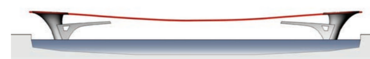
Phase 2. The suspension cables are spun across the river and tensioned to ensure they are not within the navigation zone.
