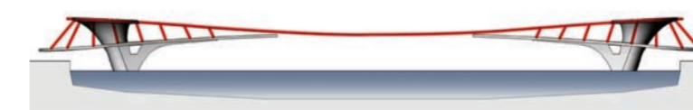
Phase 3. The lower deck is a steel arch constructed for each side towards the middle eliminating the need to obstruct the river below.
