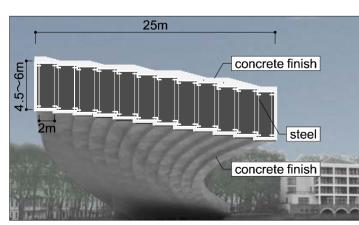
We span the bridge with simple arch beams. The steel structure member with concrete finishing can achieve the light weight of the whole bridge.
