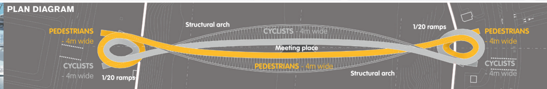
Challenge: Construction and minimal impact on river traffic SINGLE SPAN, NO PIERS IN THE RIVER
