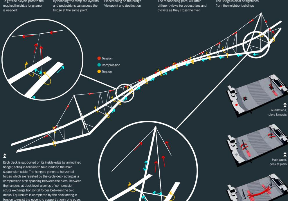
The main suspension cable acts in tension to transfer forces into
