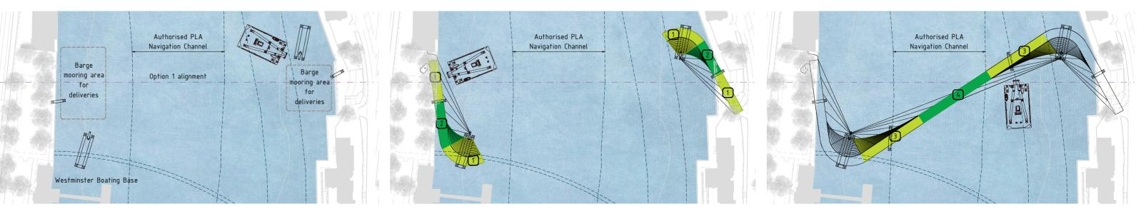
2. Temporary supports installed for north and south approach ramps and adjacent to pylons with tubular steel 3. Back span deck sections transported to site via the river and erected on temporary supports using a piled foundations to river bed. Pylons transported to site via the river and erected using a barge mounted crane. barge mounted crane. Cables installed.
